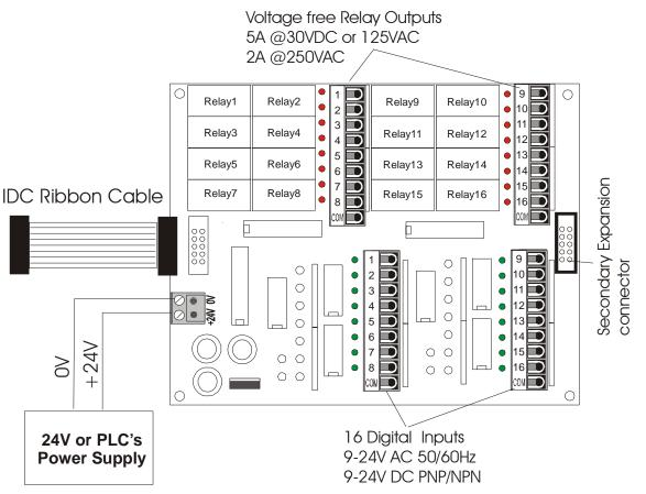
Figure 1 - 32 I/O Expansion board for FMD and F-Series PLCs
